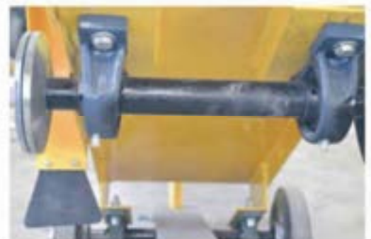
Enlarged Bearing, Reinforced Power Shaft
